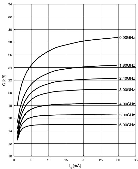
**Power gain  $G_{\text{ma}}, G_{\text{ms}} = f(V_{\text{CE}})$**
